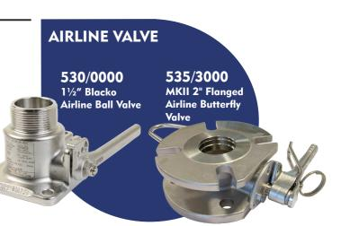
An airline valve allows the vessel to be connected to a vapour line or compressed air supply to provide vapour recovery, to purge the tank or to accelerate cargo discharge.
