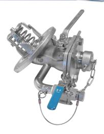
3" 45° Highlift footvalve to 2" Ball valve assembly - 8 hole inlet footvalve with replaceable seat, reducing to a 2" firesafe designed ball valve terminating in a 2" BSP outlet spigot and fitted with a 2"BSP cap. The assembly incorporates a 90° sampling point with a ¾" ball valve fitted with a nipple adaptor and ¾"BSP cap. Contact parts manufactured in 316 stainless steel with Fortyt seal to the footvalve and PTFE seals to the ball valve.
