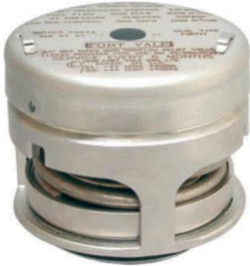
M90 x 2mm 65mm NB MK3 Super Maxi Relief Valve - M90 x 2mm threaded connection with 65mm to 80mm tapered nominal bore. Suitable for a pressure range of between 2 - 75 PSI (0.14 - 5.17 bar) and a vacuum range of between 0 - 24" Hg (0 - 0.81 bar). Contact parts manufactured in Alloy C276 with Halar coated pressure springs and Alloy C276 vacuum springs. Fitted with Fortyt seals as standard. Complete with rubber/PTFE tank seal.
