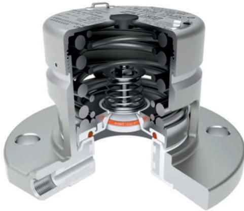
Lined 65mm NB Flanged MK3 Super Maxi Relief Valve-flange drilling to suit customer requirements (See Range) Suitable for a pressure setting of between 3 PSI to 66 PSI (0.21 to 4.55 Bar) and a vacuum setting of between 0.5"Hg to 6.2"Hg (0.02 to 0.21 Bar). Manufactured with PFA lined body, pressure plate and vacuum poppet, Halar® coated pressure spring(s) and high nickel alloy vacuum spring. Fitted with Fortyt seal as standard. May be supplied with or without gauge tapping.
