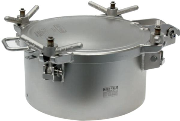
**500mm Rail Manlid Assembly** - 4 point fastening. To suit a MAWP of 3 Bar. 10mm thick x 250mm deep neckring. Contact parts manufactured in 316 stainless steel. Seal supplied separately.
