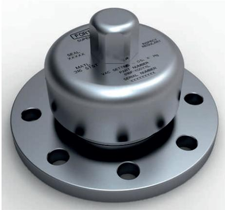
PTFE Lined 80mm NB Flanged Vacuum Vent Valve - flange drilling to suit customer requirements. (See Range) Suitable for a vacuum range of between 0.5"Hg to 6.2"Hg (0.02 Bar to 0.21 Bar) Manufactured in stainless steel fitted with Fortyt seal as standard. Wetted parts of body fitted with a PTFE liner. Poppet manufactured in high nickel alloy. Fitted with weatherproof cowl.
