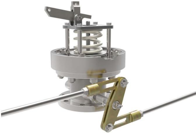
5" 180° Rail Footvalve - with dual handle assembly. Inlet flange drilled 8 x 18mm holes on a 210mm PCD. Outlet flange drilled 8 x 18mm holes on a 200mm PCD. Contact parts manufactured in 316 stainless steel. Fitted with PTFE/Elastomer main seal. Non contact parts manufactured in 304 stainless steel / mild steel.
