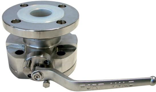
PFA Lined 50mm Full Bore Flanged Ball Valve - inlet flange drilled 4 x 18mm holes on a 126mm PCD; outlet flange drilled 4 x 18mm slots on a 120.7mm to 127mm PCD. Valve manufactured in stainless steel with PTFE main seal. All parts in contact with the cargo lined with PFA.
