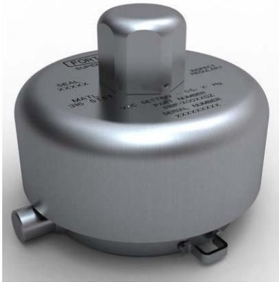
3" BSP Female Vacuum Vent Valve - suitable for a vacuum range of between 0.5"Hg to 6.2"Hg (0.02 Bar to 0.21 Bar). Manufactured in 316 stainless steel fitted with Fortyt seal. Fitted with weatherproof cowl and gauze ring.
