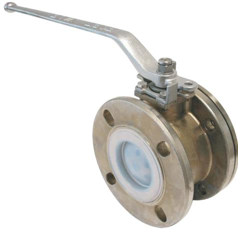
PFA Lined 80mm Full Bore Ball Valve - inlet flange drilled 4 x 18mm holes on a 160mm PCD; outlet flange drilled 4 x 18mm slots equi-spaced on a 146 to 160mm PCD. (3" BSTD to DIN80) Left hand operated with TIR to handle. Valve manufactured in stainless steel with PTFE main seal. All parts in contact with the cargo lined with PFA.
