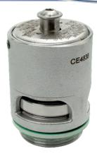
1½" BSP Twinact Relief Valve - 1½" BSP male connection. Suitable for a pressure range of between 1 to 64 PSI (0.07 to 4.41 Bar) and a vacuum range of between 0.5" to 28" Hg (0.02 to 0.94 Bar). Contact parts manufactured in 316 stainless steel fitted with Fortyt (FEP encapsulated silicone O ring) seals as standard. Complete with manual vent button and CNAF tank seal.
