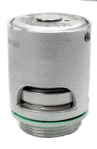
1½" BSP Twinact Relief Valve - 1½" BSP male connection. Suitable for a pressure range of between 1 to 64 PSI (0.07 to 4.41 Bar). Contact parts manufactured in 316 stainless steel fitted with Fortyt (FEP encapsulated silicone O ring) seal as standard. Complete with CNAF tank seal.
