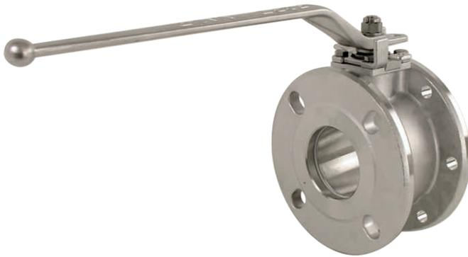
3" Blacko Ball Valve Assembly - inlet flange drilled 6 x 14mm holes on a 168mm PCD. Slotted 4 hole outlet flange. Left hand operated. Contact parts manufactured in 316 stainless steel with PTFE seals.
