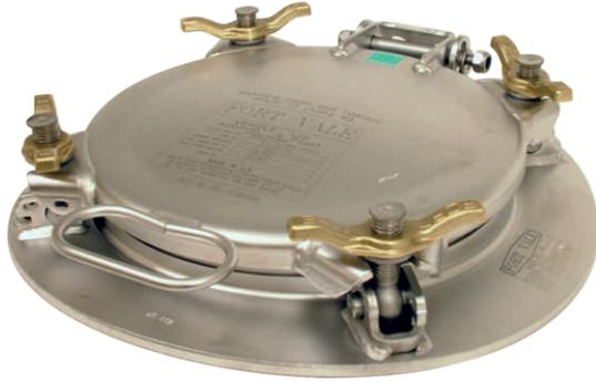
300mm Ultra Low Profile Inspection Hatch Assembly - 4 point fastening double skin cover. 8mm thick pressed neck/compensating ring profiled to suit tank radius range from 750 to 1220mm. Contact parts manufactured in 316 stainless steel. Stainless steel swingbolts with naval brass handnuts. Seal supplied separately.
