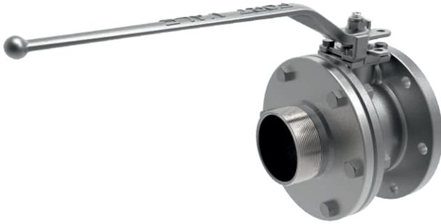
3" Blacko Ball Valve - inlet flange drilled 6 x 14mm holes (see below) on a 168.3mm PCD; 3" BSP male outlet connection. Left hand operated with TIR facility to handle. Contact parts manufactured in 316 stainless steel with PTFE seals.
