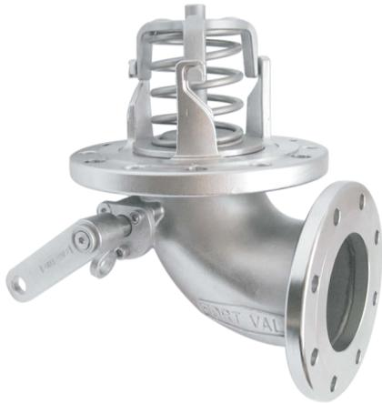
3" 90° Tankstream Footvalve - 3" to 3" 90° footvalve assembly. Inlet flange drilled 12 x 14mm holes on a 6.25" PCD. 6 inlet holes are plugged with a plastic plug. Outlet flange drilled 8 x 10.5mm holes on a 124mm PCD. Contact parts manufactured in 316 stainless steel with Fortyt or Viton O ring.
