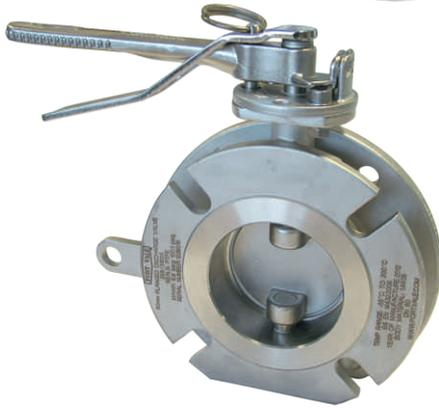
**3" Flanged Butterfly Valve** - inlet flange drilled 6 x 14mm holes spaced as shown below on a 168mm PCD; outlet flange with 4 slots 17mm equi-spaced on a 146mm PCD. Left hand operated with TIR and padlock facility to handle. Contact parts manufactured in 316 stainless steel with PTFE seals.
