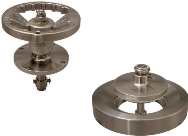
**4" Screwdown Valve** - comprising: top tank weld-in pad, stud kit and PTFE gasket; spring-loaded top operator; 4" poppet assembly with PTFE seal disc; 4" NB bottom tank weld-in pad with replaceable seat area. Contact parts manufactured in 316 stainless steel.
