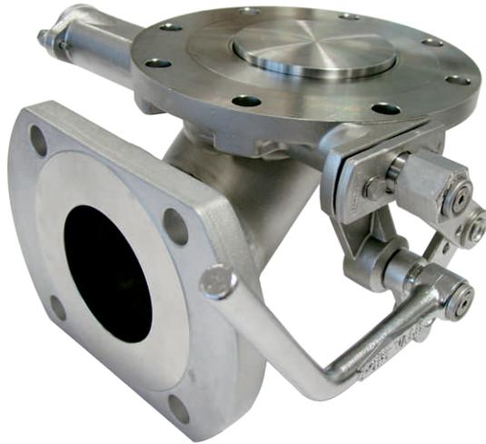
**3" 90° Cleanflow Footvalve** - inlet flange drilled 8 x 14mm holes equi-spaced on a 178mm PCD; outlet flange drilled 4 x 17mm holes equi-spaced on a 160mm PCD with flats milled top and bottom. Footvalve body with 'Superseat' (alloy 625) seating area. All other contact parts manufactured in 316 stainless steel with Fortyt O ring to main poppet as standard.
