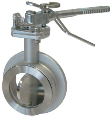
**3" Clamped Butterfly Valve** - left hand operated with TIR to handle and padlock facility. Contact parts manufactured in 316 stainless steel with PTFE main seal.
