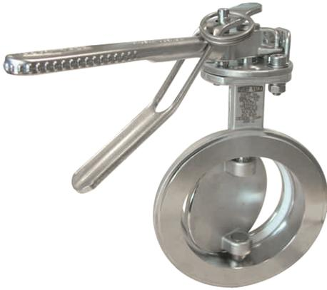
4" Clamped Butterfly Valve - left hand operated with TIR to handle and padlock facility. Contact parts manufactured in 316 stainless steel with Flexityt main seal.
