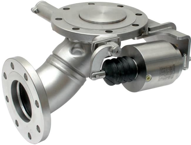
4" 90° Pneumatic Cleanflow Footvalve - inlet flange drilled 8 x 18mm holes equi-spaced on a 210mm PCD (DIN125 PN16); outlet flange drilled 8 x 18mm holes equi-spaced on a 180mm PCD (DIN100 PN16). Footvalve body with 'Superseat' (alloy 625) seating area. All other contact parts manufactured in 316 stainless steel with Fortyt O ring to main poppet as standard.
