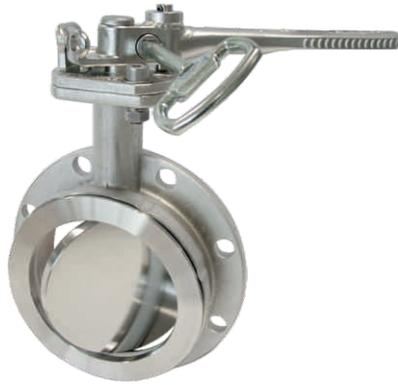
100mm Clamped Butterfly Valve - drilled TW100. Designed to clamp between two TW100 flanges with the bolts passing through the valve body holes. Left hand operated lockable handle with T.I.R. Contact parts manufactured in 316 stainless steel with Flextyt main seal.
