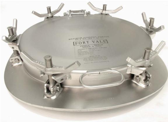
500mm Pendle Manlid Assembly - 6 point double skin manlid cover, hinged to open to 135°. Deep pressed neck/compensating ring, 51mm in height, profiled to suit a tank radius of between 850mm and 1220mm. To suit a MAWP of 3 Bar. Contact parts manufactured in 316 stainless steel with stainless steel swingbolt assemblies. Seal supplied separately.
