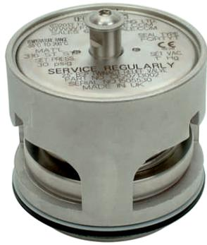
2½" BSP Twinact Relief Valve - 2½" BSP male connection. Suitable for a pressure range of between 1 to 63 PSI (0.07 to 4.34 Bar) and a vacuum range of between 0.5" to 28"Hg (0.02 to 0.94 Bar). Contact parts manufactured in 316 stainless steel fitted with Fortyt (FEP encapsulated silicone O ring) seals as standard. Complete with manual vent button and rubber/PTFE tank seal.
