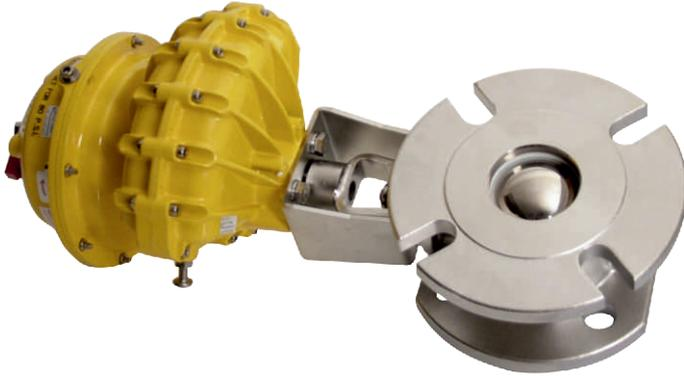
2" Pneumatically Operated Air Inlet Ball Valve - inlet flange drilled 4 x 18mm holes on a 125mm PCD; outlet flange 4 x 18mm open slots on a 120.7mm minimum PCD to suit 2" ASA 150/DIN50 PN40. Valve manufactured in 316 stainless steel with PTFE seals. Fitted with Kinetrol pneumatic actuator with spring return and 1/4" BSP air inlet.
