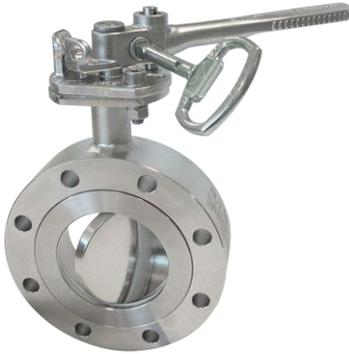
80mm Clamped Butterfly Valve - drilled TW 80. Designed to clamp between two TW80 flanges with the bolts passing through the valve body holes. Left hand operated lockable handle with T.I.R. Contact parts manufactured in 316 stainless steel with PTFE seal.
