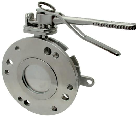
3" Flanged Butterfly Valve - inlet flange dual drilled: 6 x 14mm holes on a 168.3mm PCD and 4 x 18mm holes on a 160mm PCD. Outlet flange with 4 x 17mm open slots on a 146.1mm minor PCD. Left hand operated with TIR and padlock facility to handle. Contact parts manufactured in 316 stainless steel with PTFE main seal.
