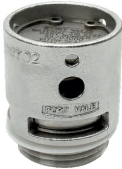
1" BSP Minnow IBC Relief Valve - 1" BSP male connection. Suitable for a pressure range of between 1 - 45 PSI (0.07 - 3.10 Bar). Contact parts manufactured in 316 stainless steel fitted with Viton seals as standard. Complete with PTFE tank seal.
