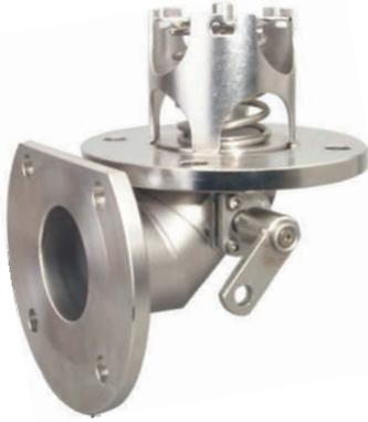
**3" 90° Highlift Footvalve** - inlet flange drilled 4 x 18mm holes on a 160mm PCD; outlet flange drilled 4 x 18mm holes on a 160mm PCD with flat milled at 72mm to horizontal centre line. Contact parts manufactured in 316 stainless steel with Fortyt O ring to main poppet as standard.
