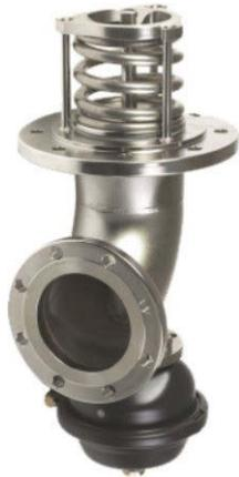
4" 90° Pneumatic "Sealty" Extended Footvalve - inlet flange drilled 8 x 14mm holes equi-spaced on a 190mm PCD; outlet flange drilled 8 x 14mm holes equi-spaced on a 150.1mm PCD. Manufactured in 316 stainless steel with elastomer core PTFE main seal.
