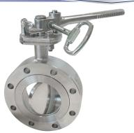
80mm Clamped Butterfly Valve - drilled TW 80. Designed to clamp between two TW80 flanges with the bolts passing through the valve body holes. operated lockable handle with T.I.R. Contact parts manufactured in 316 stainless steel with PTFE seal.
