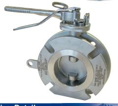
3" Flanged Butterfly Valve - inlet flange drilled 6 x 14mm holes spaced as shown below on a 168mm PCD; outlet flange with 4 slots 17mm equi-spaced on a 146mm PCD. Left hand operated with TIR and padlock facility to handle. Contact parts manufactured in 316 stainless steel with PTFE seals.
