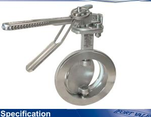
4" Clamped Butterfly Valve - left hand operated with TIR to handle and padlock facility. Contact parts manufactured in 316 stainless steel with Flextyt main seal.
