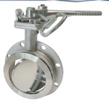
100mm Clamped Butterfly Valve - drilled TW100. Designed to clamp between two TW100 flanges with the bolts passing through the valve body holes. Left hand operated lockable handle with T.I.R. Contact parts manufactured in 316 stainless steel with Flextyt main seal.
