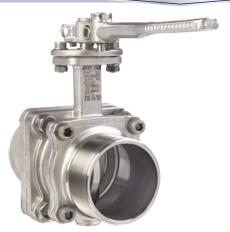
3" NB Tank-Pro Butterfly Valve - weld-prepared inlet and 3"BSP threaded outlet. Lockable handle with T.I.R. as standard. Contact parts manufactured in 316 stainless steel with PTFE main seal.
