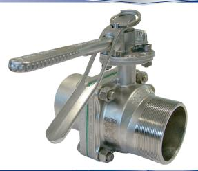
3" Unifly Road Tanker Butterfly Valve - weld-prepared inlet and 3" BSP threaded outlet. Contact parts manufactured in 316 stainless steel with PTFE main seal.
