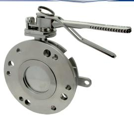
3" Flanged Butterfly Valve - inlet flange dual drilled: 6 x 14mm holes on a 168.3mm PCD and 4 x 18mm holes on a 160mm PCD. Outlet flange with 4 x 17mm open slots on a 146.1mm minor PCD. Left hand operated with TIR and padlock facility to handle. Contact parts manufactured in 316 stainless steel with PTFE main seal.
