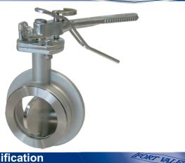
3" Clamped Butterfly Valve - left hand operated with TIR to handle and padlock facility. Contact parts manufactured in 316 stainless steel with PTFE main seal.
