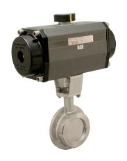
3" Clamped Butterfly Valve with Spring Return Pneumatic Actuator - valve connection to actuator to ISO 5211 / DIN 3337 standards. Counter-clockwise opening. Contact parts manufactured in 316 stainless steel with PTFE seal.
