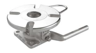
11/2" Flanged Airline Ball Valve - inlet flange slotted to 11/2" BSTD/11/2" ASA 150. Complete with pressure gauge connection, gauge guard and TIR facility to handle. Contact parts manufactured in 316 stainless steel with PTFE seals.
