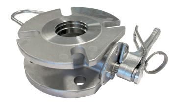
2" Flanged Airline Butterfly Valve - inlet flange slotted to suit 2" BSTD minimum. 4 hole tank connection to DIN50 PN10. Complete with ½"BSP pressure gauge connection, gauge guard and TIR facility to handle. Contact parts manufactured in 316 stainless steel with PTFE seals.
