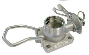
2" Airline Butterfly Valve - 2" BSP male inlet. Complete with pressure gauge connection, gauge guard and TIR facility to handle. Contact parts manufactured in 316 stainless steel with PTFE seals.
