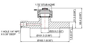
This assembly is suitable for gas phase applications.
