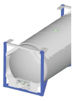
ISO Liquefied Gas Tank Container Equipment
