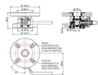
PFA Lined 25mm Reduced Bore Flanged Airline Ball Valve - inlet flange drilled 4 x 18mm slots on a 100mm to 125mm PCD; outlet flange (tank connection) drilled 4 x 11mm holes on a 103.5mm PCD. Valve manufactured in stainless steel with PTFE main seal. All parts in contact with the cargo lined with PFA.
