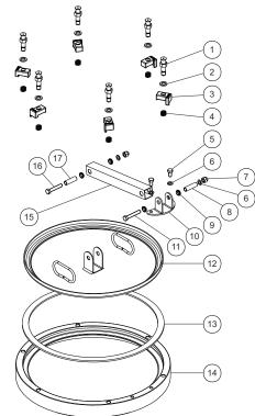
500mm Side Entry Manlid Assembly - suitable for Milk Tankers. Cover with cross arm and 6 point fastening with clamp system. 60mm deep neckring. Contact parts manufactured in 304 stainless steel. Fitted with a sweet white rubber seal. (FDA compliant)
