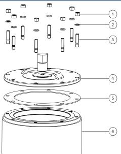
300mm Flash Vacuum Vent Assembly - Allows an emergency flow of air into the vessel to protect it from vacuum damage, for example during CIP.
