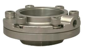
The burst disc adaptor assembly is designed to hold a 65mm/65mm XL burst disc between the tank and a  $2\frac{1}{2}$ " BSP relief valve. It is designed for use in conjunction with the Fort Vale manometer to monitor the integrity of the disc. (Burst disc not included)
