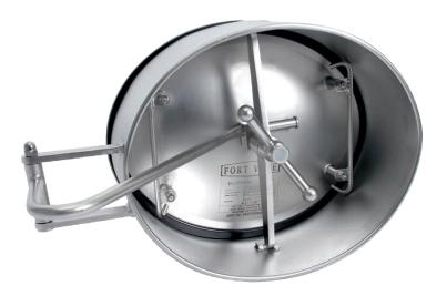
In/Out Oval Manlid Assembly with Deep Neckring - to suit Hygienic applications. 405.5mm x 507mm assembly with 200mm deep x 10mm thick neckring. Contact parts manufactured in 316 stainless steel polished to 180 grit. Cover fitted with vulcanised Blue Nitrile seal.
