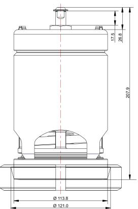
65mm NB Foodgrade Extended Body Relief Valve with 100mm DIN11851 connection - Designed and tested for incompressible fluid flow. Suitable for a pressure range of between 3 - 50 PSI (0.21 - 3.45 Bar) and a standard vacuum setting of 0.5"Hg (0.02 Bar). Contact parts manufactured in 316 stainless steel. Fitted with Fortyt and EPDM seals.
