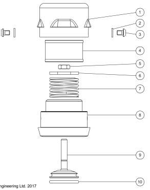
11/2" Vacuum Only Uniact Relief Valve with 50mm DIN11851 connection - Suitable for a vacuum range of between 0.5"Hg and 22"Hg (0.02 Bar and 0.75 Bar). Single-acting valve - vacuum relief only. Contact parts manufactured in 316 stainless steel fitted with Fortyt seal (FEP encapsulated silicone O ring) as standard. Supplied with stainless steel gauzed cap. 50mm DIN 11851 nut and seal supplied separately.
