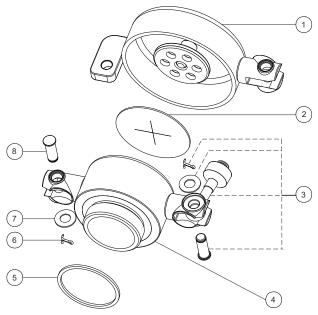
2"BSP Highflow Milk Breather Vent Valve - has a male screw connection and a hinged cap, enabling easy removal of the cap or the complete valve for inspection, cleaning and seal replacement. The cap can be opened by releasing the swingbolt. The valve has a food-grade silicone membrane seal which allows passage of air under pressure or vacuum conditions whilst preventing escape of liquid product during transit. Contact parts manufactured in 316 stainless steel.
