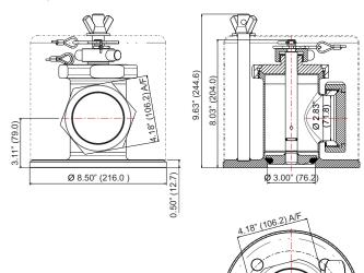
4 HOLES Ø 0.71" (18.0) EQUI-SPACED ON A \_\_\_\_\_ 6.00" (152.4) PCD (3" ANSI 150)
