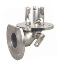
3" 90° Highlift Footvalve - inlet flange drilled 4 x 18mm holes on a 160mm PCD; outlet flange drilled 4 x 18mm holes on a 160mm PCD with flat milled at 72mm to horizontal centre line. Contact parts manufactured in 316 stainless steel with Fortyt O ring to main poppet as standard.
