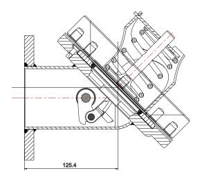
N.B. Above dimension is for a standard 45° valve and will vary according to valve specification
