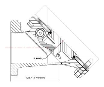
N.B. Above dimension is for a standard 45° valve and will vary according to valve specification
