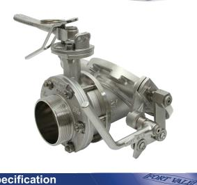
3" 45° Composite Bottom Outlet Assembly - comprising of 3" Cleanflow Footvalve bolted through the 3" Clamped Butterfly valve terminated with a 3" BSP outlet flange. Butterfly valve is left hand operation. Contact parts manufactured in 316 stainless steel with Fortyt main seal to footvalve and PTFE main seal to butterfly valve.
