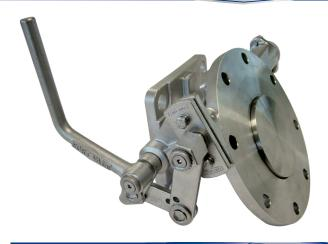
holes equi-spaced on a 178mm PCD; square outlet flange drilled 4 x 17mm holes on a 160mm PCD. Contact parts manufactured in 316 stainless steel with Fortyt O ring to main poppet as standard.
