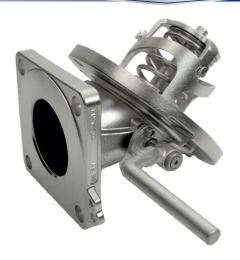
3" 45° MKIII Highlift Footvalve - inlet flange drilled 8 x 14mm holes equi-spaced on a 178mm PCD; outlet flange drilled 4 x 17mm holes on a 160mm PCD. Footvalve body with 'Superseat' (alloy 625) seating area. All other contact parts manufactured in 316 stainless steel. Fitted with a Fortyt poppet O ring.
