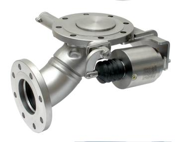
4" 90° Pneumatic Cleanflow Footvalve - inlet flange drilled 8 x 18mm holes equi-spaced on a 210mm PCD (DIN125 PN16); outlet flange drilled 8 x 18mm holes equi-spaced on a 180mm PCD (DIN100 PN16). Footvalve body with 'Superseat' (alloy 625) seating area. All other contact parts manufactured in 316 stainless steel with Fortyt O ring to main poppet as standard.
