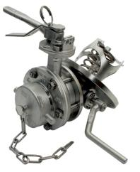
3" 45° Composite Bottom Outlet Assembly - comprising of a 3" 45° Highlift footvalve, 3" clamped butterfly valve and a 3" BSP eccentric outlet flange with stainless steel cap and PTFE washer. The assembly includes the butterfly valve intermediate gasket and the footvalve/butterfly valve bolting kit. Contact parts manufactured in 316 stainless steel with a Fortyt Footvalve main seal and a PTFE butterfly valve main seal.
