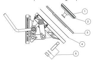
IMPORTANT NOTE: When fitted with the replaceable seat, the Footvalve will protrude further and the outlet centre line will be lower than that of a standard Footvalve. Please contact our Sales team for more detailed information.
