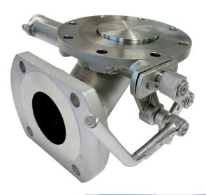
3" 90° Cleanflow Footvalve - inlet flange drilled 8 x 14mm holes equi-spaced on a 178mm PCD; outlet flange drilled 4 x 17mm holes equi-spaced on a 160mm PCD with flats milled top and bottom. Footvalve body with 'Superseat' (alloy 625) seating area. All other contact parts manufactured in 316 stainless steel with Fortyt O ring to main poppet as standard.
