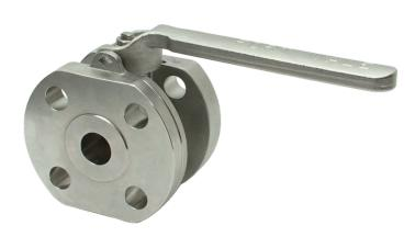
1" Full Bore Firesafe / Lethal Service Ball Valve - inlet and outlet flange drilled 4 x 18mm holes equi-spaced on a 89mm PCD. Contact parts manufactured in 316 stainless steel fitted with TFM PTFE main seal.
