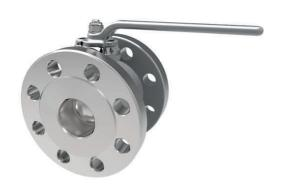
2" Full Bore Firesafe / Lethal Service Ball Valve - inlet and outlet flange drilled 8 x 19mm holes equi-spaced on a 127mm PCD (2" ASA 300). Contact parts manufactured in 316 stainless steel fitted with TFM PTFE main seal.
