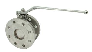
3" Full Bore Firesafe / Lethal Service Ball Valve - inlet and outlet flange drilled 8 x 18mm holes equi-spaced on a 160mm PCD. Contact parts manufactured in 316 stainless steel fitted with TFM PTFE main seal.
