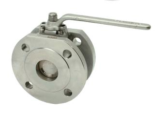
2" Full Bore Firesafe Ball Valve - inlet and outlet flange drilled 4 x 18mm holes equi-spaced on a 125mm PCD. Contact parts manufactured in 316 stainless steel fitted with TFM PTFE main seal.
