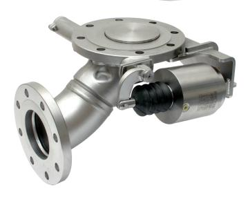
4" 90° Pneumatic Cleanflow Footvalve - inlet flange drilled 8 x 18mm holes equi-spaced on a 210mm PCD (DIN125 PN16); outlet flange drilled 8 x 18mm holes equi-spaced on a 180mm PCD (DIN100 PN16). Footvalve body with 'Superseat' (alloy 625) seating area. All other contact parts manufactured in 316 stainless steel with Fortyt O ring to main poppet as standard.
