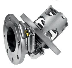
4" 45° Highlift Footvalve with Hydraulic Actuator - inlet flange drilled 8 x 18mm holes equi-spaced on a 210mm PCD (DIN125 PN10). Outlet flange drilled 8 x 18mm holes equi-spaced on a 180mm PCD (DIN100 PN10). Footvalve body with 'Superseat' (alloy 625) seating area. All other contact parts manufactured in 316 stainless steel, fitted with a Fortyt main seal. Fitted with a hydraulic actuator with 1/8" BSP connection.
