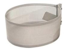
A clamped gauze ring fits around the valve body ports and offers flame protection on valves with a vacuum setting of 0.21 Bar (6"Hg) and above. For valves with a vacuum setting of less than 0.21 Bar, a clamped gauze is often fitted to offer dust protection.
