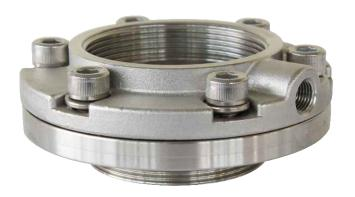
The burst disc adaptor enables a 2½"BSP female threaded tank socket, reference 600/1000, to receive a burst disc and a threaded valve. Contact parts manufactured in 316 stainless steel.
