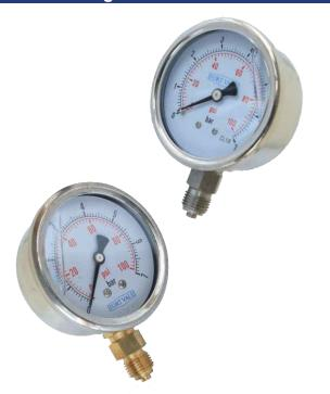
The pressure gauge fits into the relief valve flange gauge connection and provides a tank pressure reading. Where it is fitted onto a valve mounted in series with a burst disc, it may be used to detect the burst disc integrity. ½"BSP connection. Pressure range available from 0 to 20 Bar (0 to 290 PSIG).
