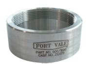
Heavy-duty tank weld-in socket with over-size thread to alleviate the need for re-tapping after welding. Available in 1½" BSP and 2½"BSP. Contact parts manufactured in 316 stainless steel.
