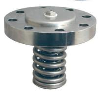
MKII 80mm Internal Gas Relief Valve - Suitable for a pressure range of between 100 - 525.5 PSI (6.90 - 36.24 Bar). Contact parts manufactured in 304/316 stainless steel. Fitted with PTFE seals as standard.
