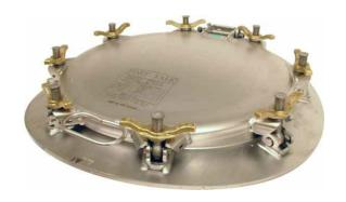
500mm Ultra Low Profile Manlid Assembly - 8 point fastening. 8mm thick pressed neck/compensating ring profiled to suit tank radius. Contact parts manufactured in 316 stainless steel. Stainless steel swingbolts with naval brass handnuts. Seal supplied separately.
