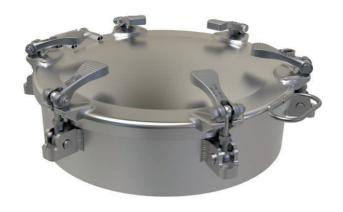
500mm Manlid Assembly with Quick Release Latches pressed 6 point fastening cover. 6mm thick x 180mm deep neckring. Contact parts manufactured in 316 stainless steel. Fitted with stainless steel quick release latches. Seal supplied separately.
