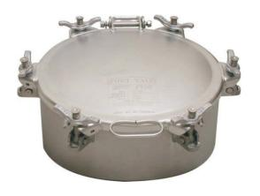
460mm Pennine Manlid Assembly - 6 point double skin cover, hinged to open to 135°. 6mm thick x 100mm deep neckring. Contact parts manufactured in 316 stainless steel with stainless steel swingbolts and handnuts. Seal supplied separately.
