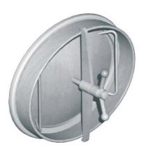
Internal Oval Manlid Assembly - opens into the tank vessel. The manlid is operated using a double arm lever and incorporates a cross arm to clamp and seal the cover on closure. Internal tank pressure enhances sealing performance. Manufactured in 316 stainless steel, internal surfaces polished to 180 grit. Fitted with sweet white rubber seal as standard.
