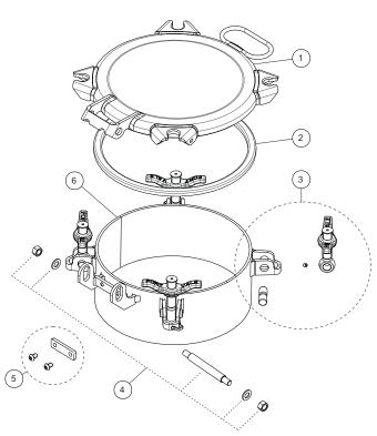
300mm Inspection Hatch - 4 point fastening. Double skin cover. 6mm thick x 100mm deep neckring. Contact parts manufactured in 316 stainless steel. Stainless steel swingbolts with naval brass handnuts. Seal supplied separately.
