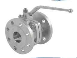
2" Full Bore Gas Ball Valve - DN 50 PN 40 high pressure valve. Flange drilling: 4 x 18mm holes on a 127mm PCD (2" ASA150) and 8 x 18mm holes on a 127mm PCD (2" ASA 300). Right hand operation. Contact parts manufactured in 316 stainless steel with PTFE seals.
