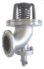
Halar Lined 4" to 3" Hydraulic Highlift Footvalve - inlet flange drilled 8 x 14mm holes equi-spaced on a 184mm PCD (4" TTMA). Outlet flange drilled 8 x 11mm holes equi-spaced on a 124mm PCD (3" TTMA). Hydraulic actuator with 1/8" NPT connections. Valve manufactured in 304/316 stainless steel fitted with a Viton main seal. All parts in contact with the cargo lined with Halar and lifting rod encased in PTFE bellows.
