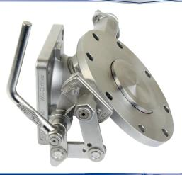
3" 45° Cleanflow Footvalve - inlet flange drilled 8 x 14mm holes equi-spaced on a 178mm PCD; outlet flange drilling as shown below. Footvalve body with 'Superseat' (alloy 625) seating area. All other contact parts are manufactured in 316 stainless steel. Fitted with a Fortyt poppet O ring.
